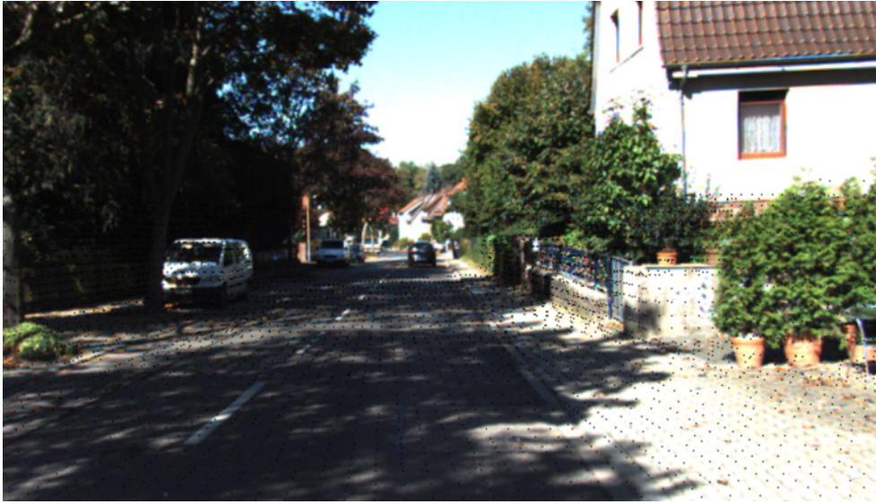
Figure 4.4: Occupied voxels projected into the image as black dots for debugging purposes.
