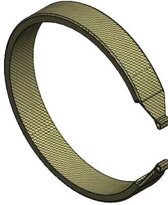
Figure 8.3: 3D representation of the modelled band.
