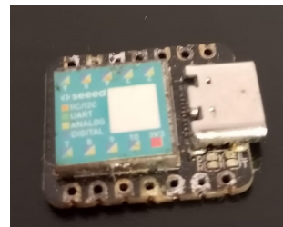
Figure 6.8: Seeduino XIAO [82] and hardware pinout [83].
