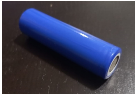
Figure 5.13: Rechargeable cylindrical lithium ion battery with 2,200 mAh capacity [64].
