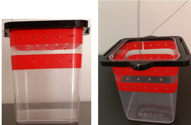
Figure 7.4: Bait holder with bottom piece clamped and bottom piece with string tied.
