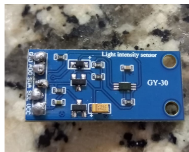
Figure 6.5: Digital Light Intensity Sensor Module BH1750FVI [75].
