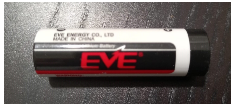
Figure 5.4: Battery with 2,700 mAh of capacity [59].
