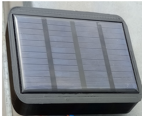
Figure 7.5: Lid with PV panel attached.
