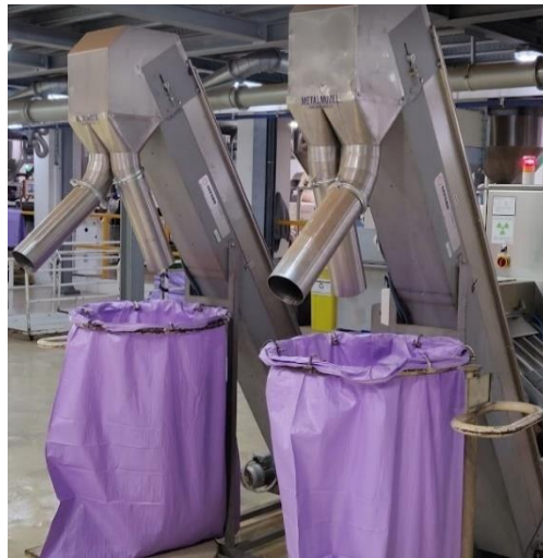
Figure 34 - Conveyor responsible to transport the stoppers to the bags
