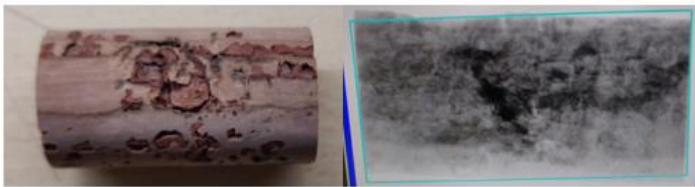
Figure 33 - Cork stopper with clay and respective X-ray image
