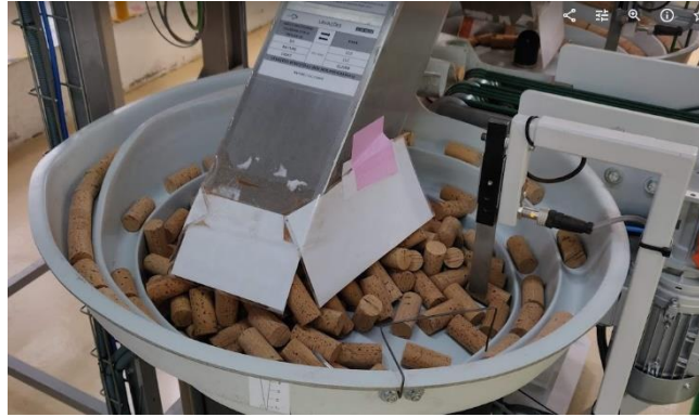
Figure 52 - Inverted V system clogged
