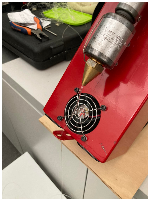
Figure 3.10: Continuous filament of PLA being extruded.
