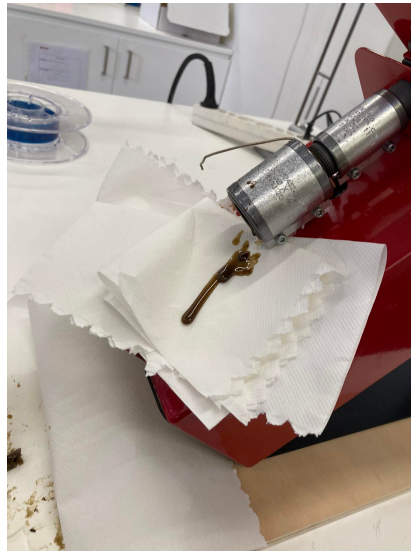
Figure 3.8: Extruder without the nozzle and material removal.
