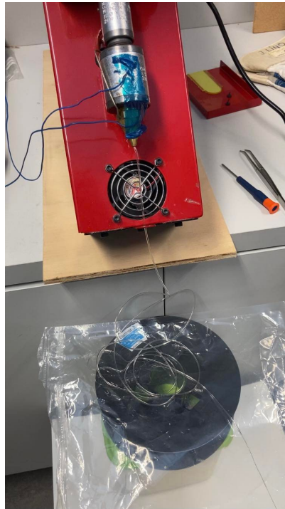
Figure 3.11: Test of PLA (97wt%) with colophony (3wt%).
