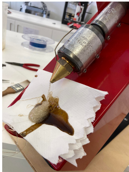
Figure 3.9: Cleaning the nozzle by adding PLA to the extruder.
