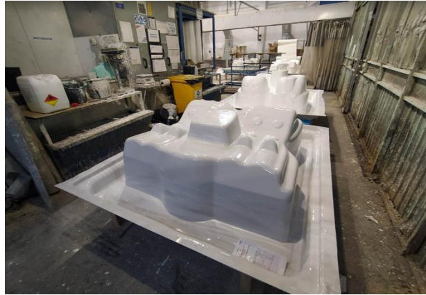
Figure 12 - Spas with epoxy resin in the preparing stage.
