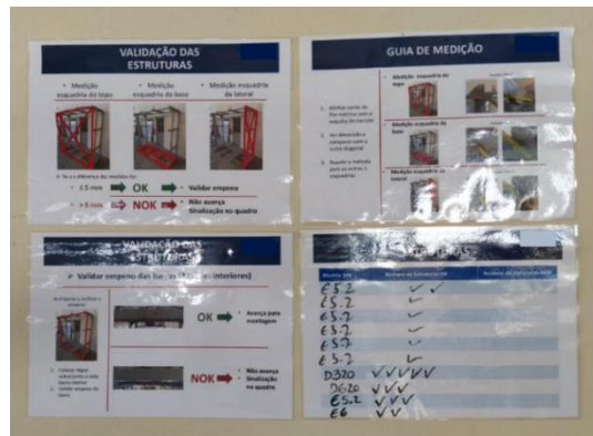
Figure 39 - Standard of Work of structures validation
