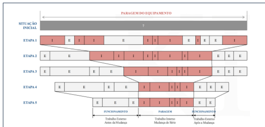
Figure 7 - The 5 steps of SMED (single-minute exchange of dies)
