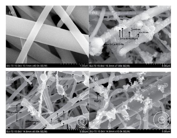
Figure 3. SEM imagens of (a) control blank quartz filter with 1.0 µm scale; (b–d) collected particles.
