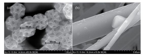
Figure 5. SEM imagens of (a) brochosomes, and (b) salt (NaCl) particles in indoor samples.
