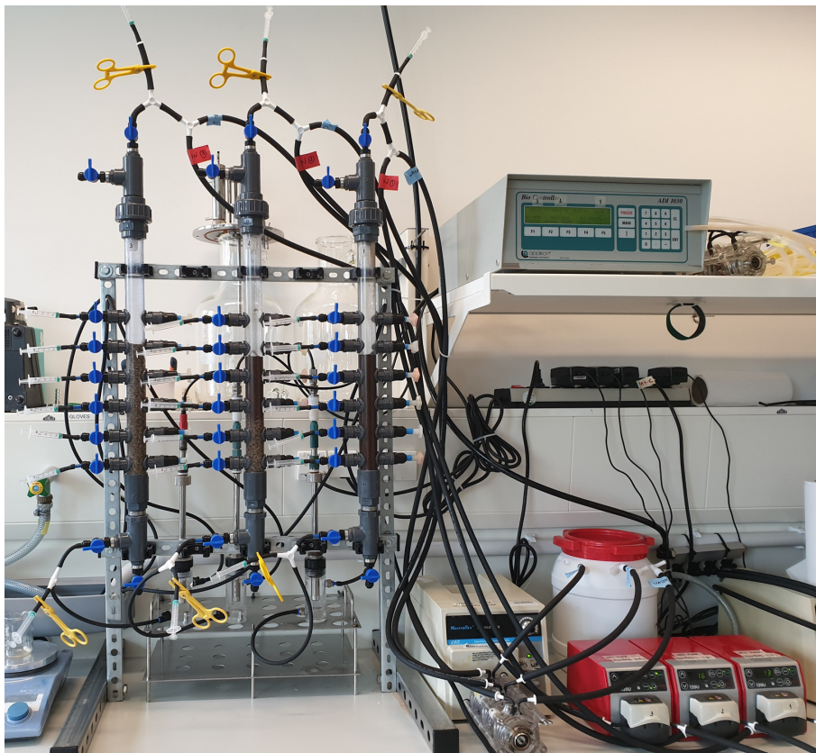
Figure 3.2: Lab-scale rapid sand filtration columns used throughout this Thesis.
