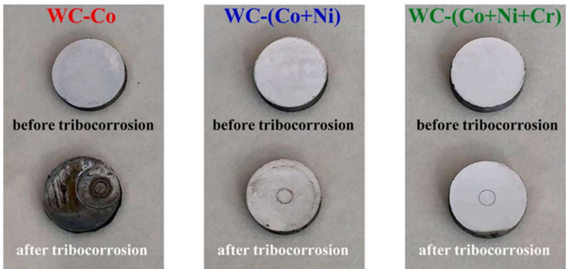
Figure 11 - Optical photograph of the cemented carbides of WC-Co, WC-(Co-Ni), and WC-(Co-Ni-Cr) taken both before and after the tribocorrosion tests in highly alkaline wet media (pH~13.65). The circle visible at the surface after the tribocorrosion tests is the corresponding residual wear track [38].
