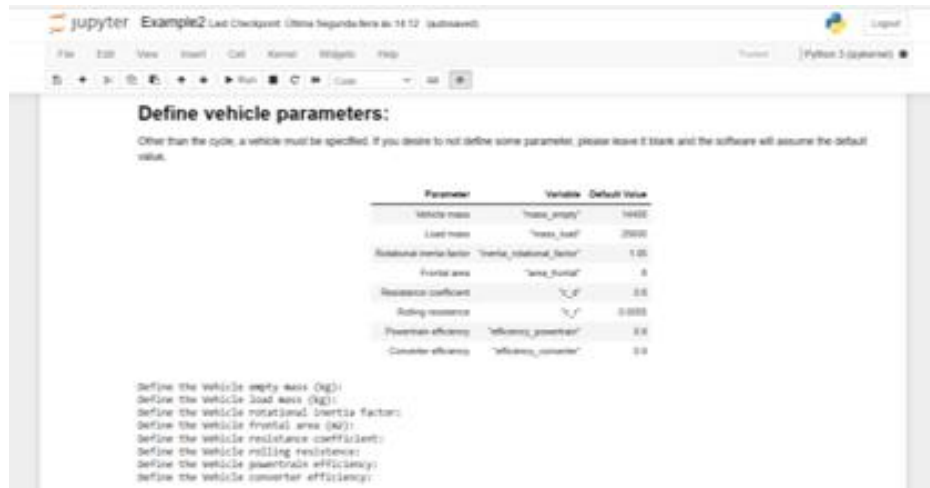
Figure E.2. User interface regarding the vehicle simulation.
