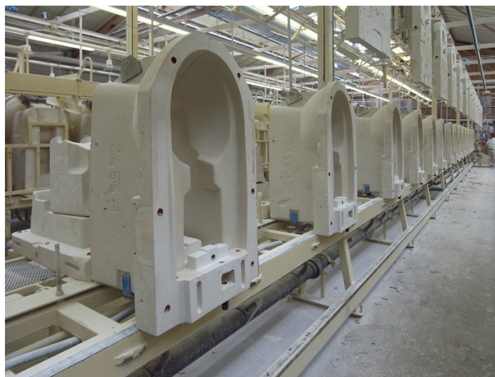
Figure 3.4: Moulds in a Production Stand
