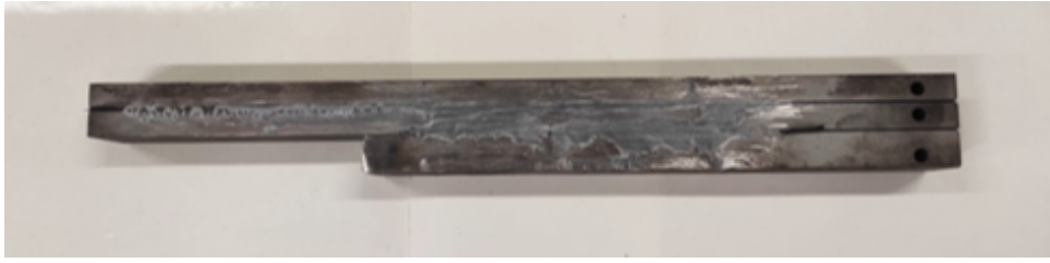
Figure 16: Manufactured unified specimen for mode I and mode II adhesive characterisation.
