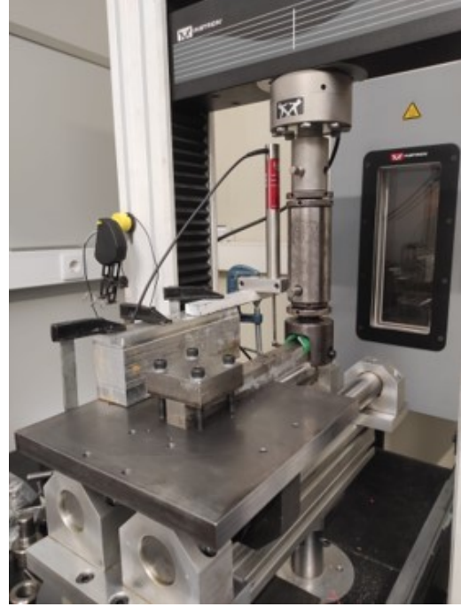
(b) LVDT to measure relative \delta .
