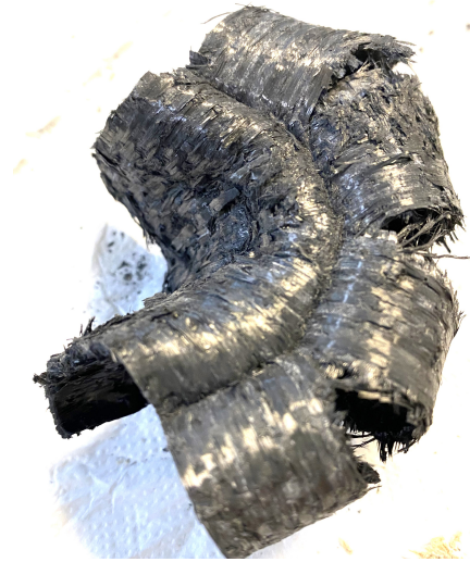
Figure 3.32: Crushed TC-3HS-1 coupon with the debris wedge removed post mortem.
