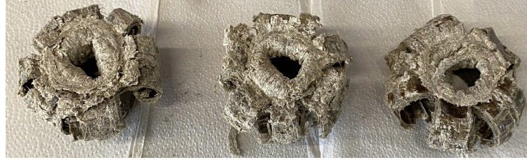
(a) All TF-2 crushed tubes.
