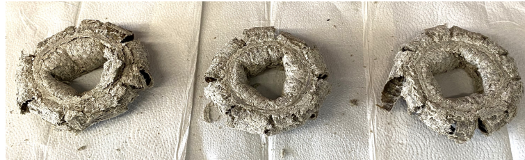
(c) All TF-4 all crushed tubes.
