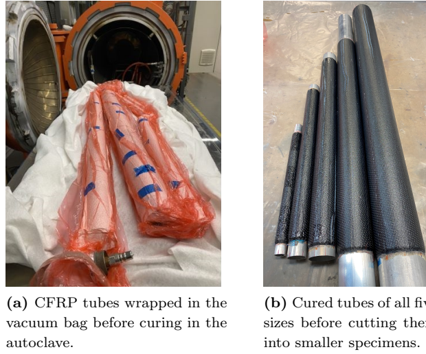
Figure 3.4: Curing of the tubular coupons.
