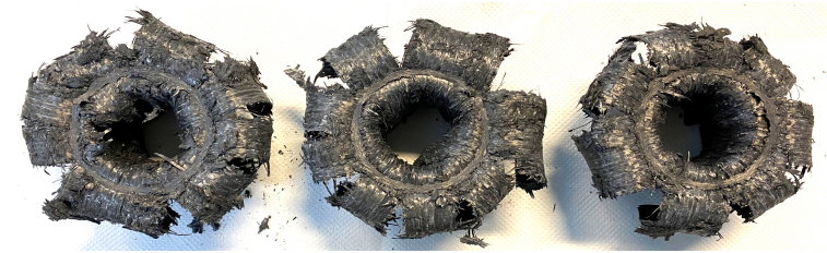
(c) All TC-3 all crushed tubes.
