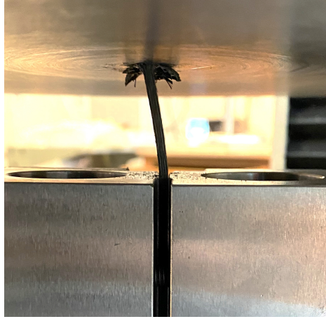
Figure 3.20: A frame from the FC-35 coupon crush test in which buckling can be observed.
