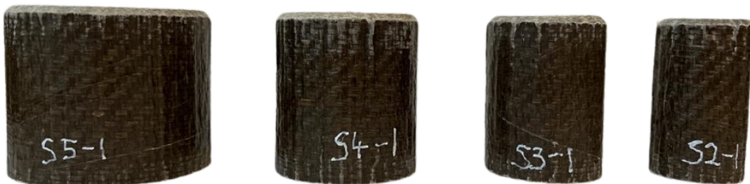
Figure 3.10: The 4 different FFRP tube sizes tested. In order from left to right: TF-5, TF-4, TF-3 and TF-2
