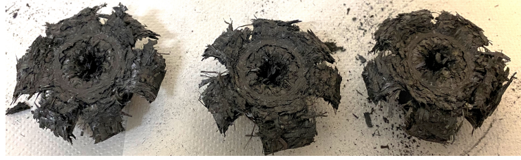
(a) All TC-1 crushed tubes.
