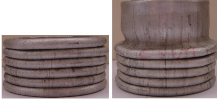
Figure 2.3: Two axially crushed tube-shaped aluminium alloy specimens (adapted from [30]).
