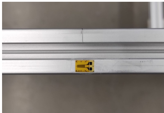
Figure 4.4: Selected HBM 1-LY43-3/120 foil strain gauge installed in the upper central member.
