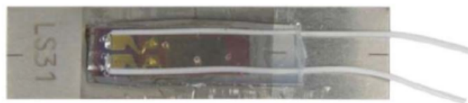
Figure 2.3: LS31 weldable strain gauge distributed by HBM [2].
