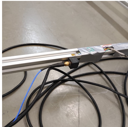
Figure 4.8: PCB Piezotronics accelerometer mounted on the structure.
