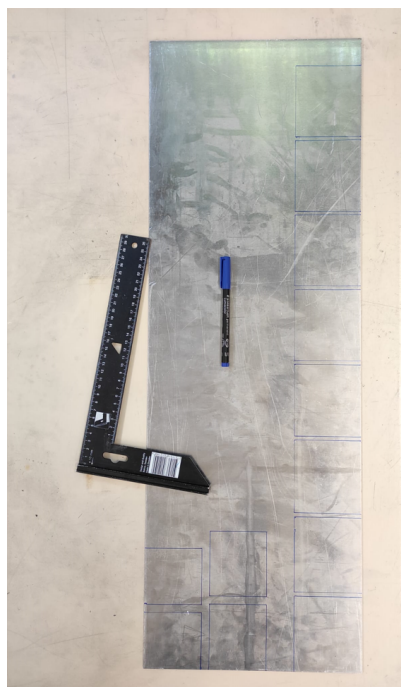
Figure 3.12: Gusset plates' contours made on the thinner aluminium sheet.
