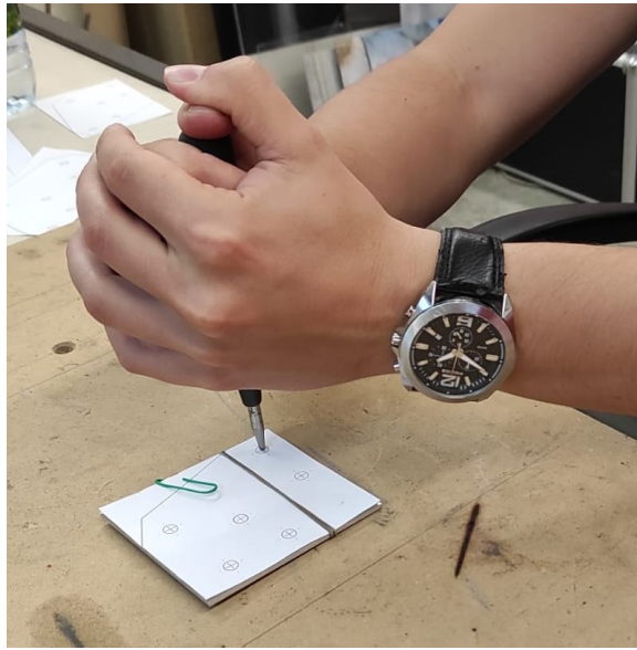
Figure 3.14: Centering punch process showing the fixation method of the drawing to the aluminium plate.
