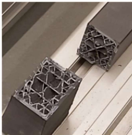
Figure 3.6 - Additive manufacturing fill analysis.
