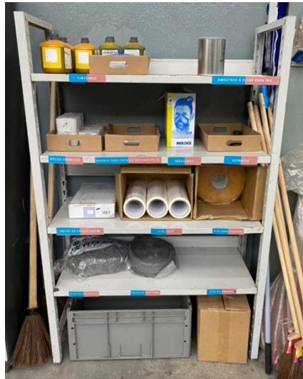
Figure 24- Consumables area after 5S implementation
