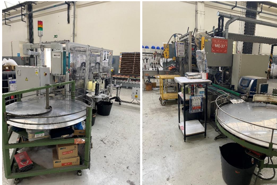
Figure 9- Automatic Filling Line composed by RO-11 and ME-37
