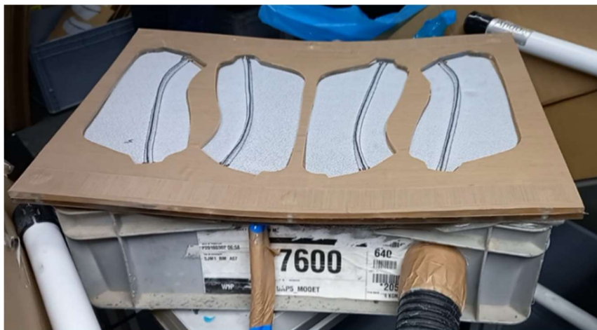
Figure 53 - Change of the process of stapling the nappa pieces to the cardboard.
