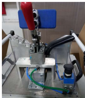
Figure 24 - Tool for the removal of the excess material of the plastic parts.
