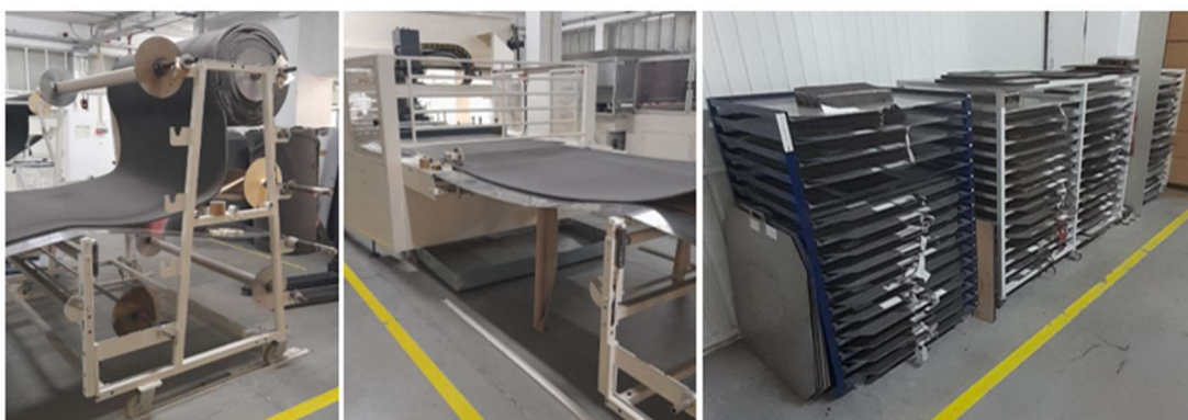
Figure 13 - Foam roll placed in the press in the left and centre. Shelf with the cutters on the right.
