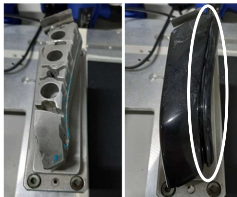
Figure 26 - Metal support for the piece on the left. Piece placed in the support with a circle around the groove for the alignment on the right.
