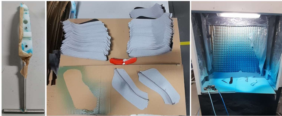
Figure 25 - Support for the plastic part on the left. Sewn nappa pieces stapled to the cardboard sheet on the centre. Glue workstation on the right.
