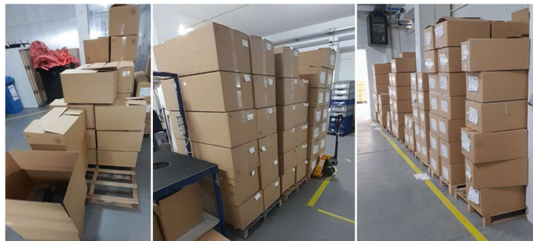
Figure 20 - Excess of WIP between the cutting press and the drills removal.
