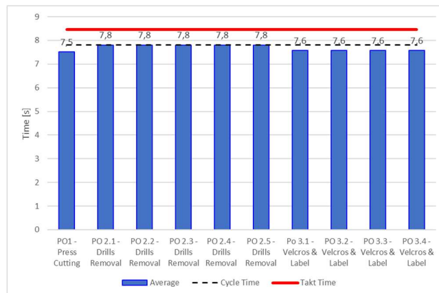
Figure 34 - Balance of the production line after calculating the correct number of operators.
