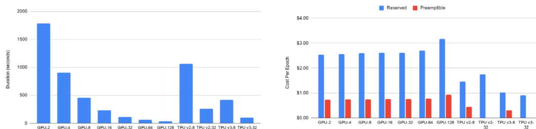
Figure 2.4: (left) The impact of increasing number of total GPUs assigned to workers on time to process one epoch of training. (right) Cost of running one epoch on the Google Cloud Platform, with Reserved vs. Preemptible resources. As explored in [22]
