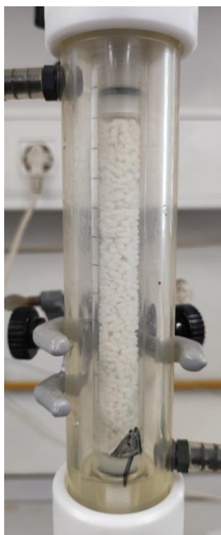
Figure 32. Packed column with pellets of MFI (H).
