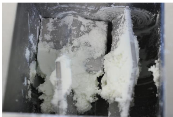
Figure 26. Sample P1 composed with 30 wt% of alumina and 0.65 mL H 2 O per gram of solid.
