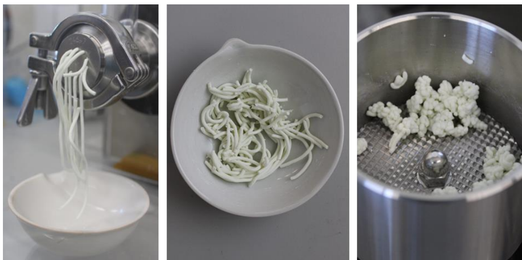
Figure 27. Sample P2 composed with 30 wt% of alumina and 0.55 mL H 2 O per gram of solid.
