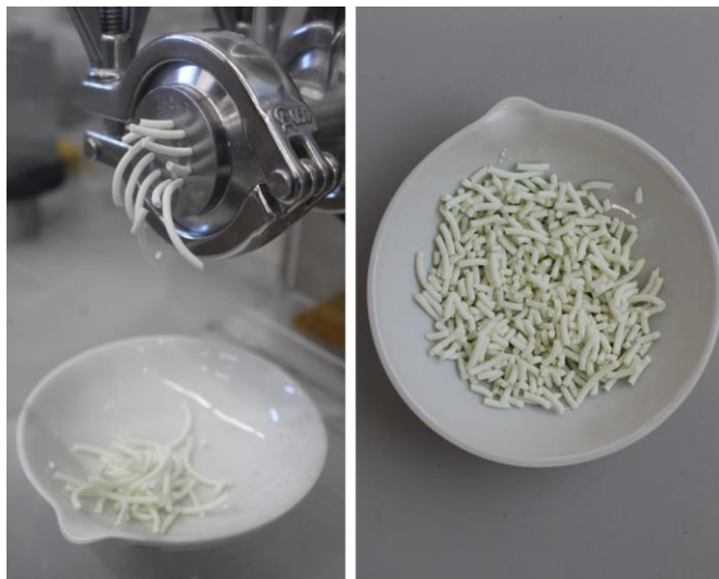
Figure 28. Sample P3 composed with 30 wt% of alumina and 0.45 mL H 2 O per gram of solid.
