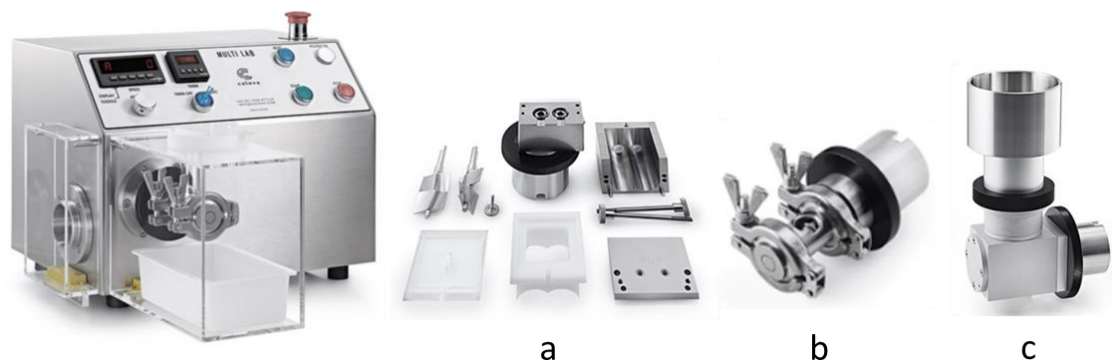
Figure 10. Caleva Multi Lab Extruder and the pieces of equipment: (a) mixing chamber, (b) extruder, and (c) spheronizer. Adapted from [44].
