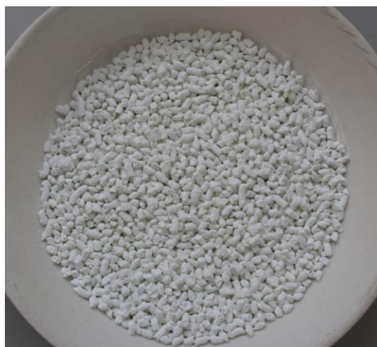
Figure 29. Sample P4 composed with 30 wt% of alumina and 0.44 mL H 2 O per gram of solid.
