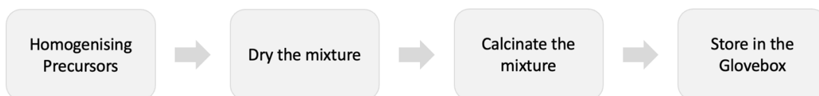
Figure 3.2 - Guidelines to cathode synthesis by solid-state reaction.
