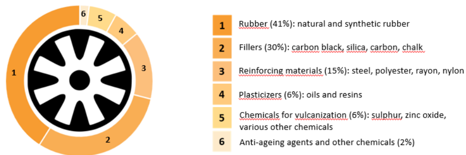
Figure 3. Composition of a modern tire. Adapted from (Continental, 2013 / 2014).
