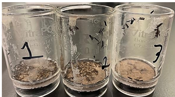
Figure 25. Result of filtrating the Cokoon dipped Rayon, dissolved for 60 minutes (1), 90 minutes (2), and 120 minutes (3).
