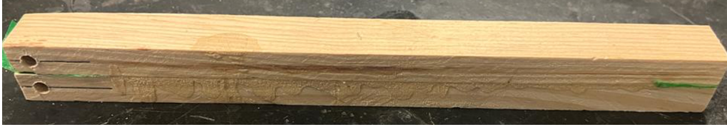
Figure 30: DCB specimen produced.
