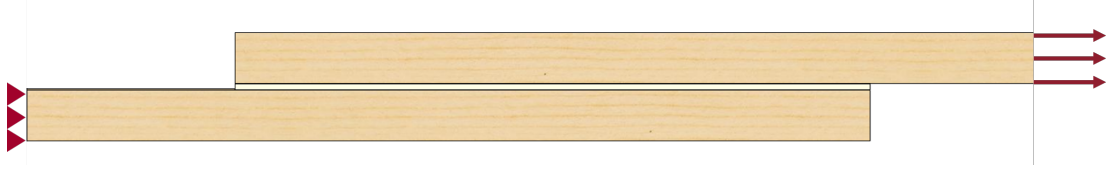
Figure 24: Illustration of the boundary conditions applied.
