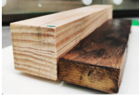
Figure 6: Visual comparison between a natural block and a densified block (with mould).
