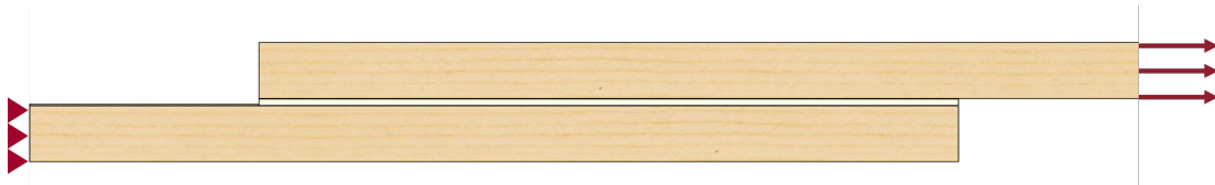
Figure 36: Illustration of the boundary conditions applied.
