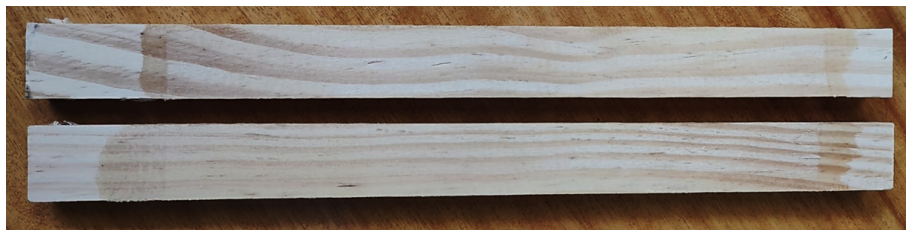
Figure 42: Fracture surfaces - DCB.
