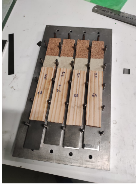
Figure 26: Mould used for the fabrication of single lap joints.
