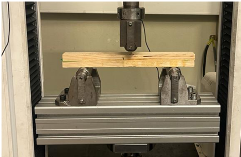
Figure 32: ENF specimen testing setup.
