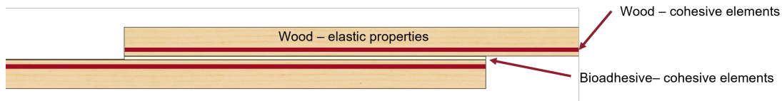
Figure 35: Illustration of the numerical model.
