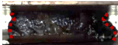
(a) Deformation of the walls under compression.
