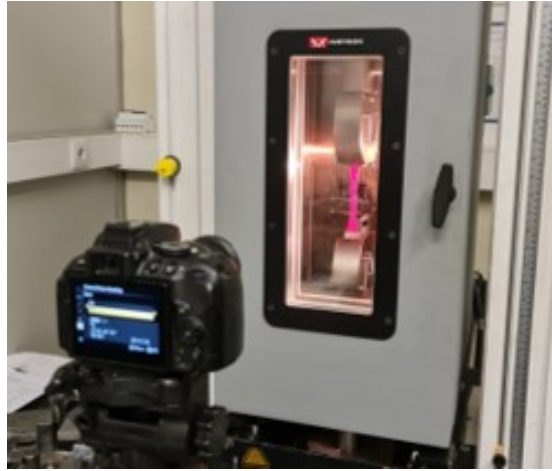
Figure 26: Tensile test setup for high temperature [50 °C].
