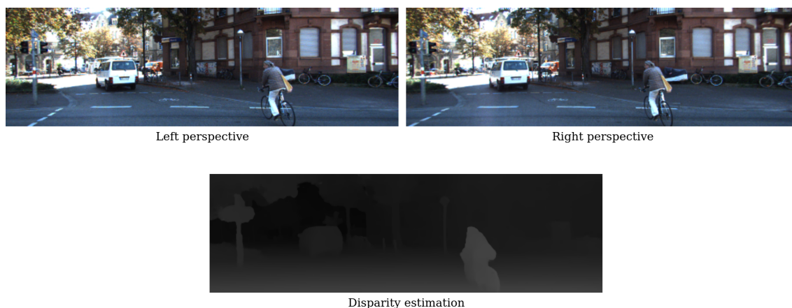
Figure 3.2: Example of a disparity estimate from PSM-Net in grayscale format; the left and right perspectives were used as inputs [80].
