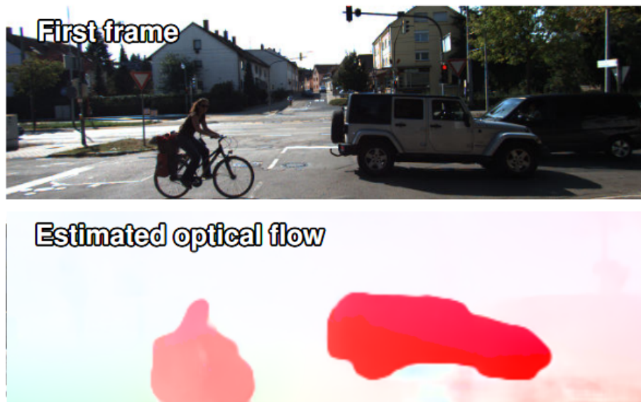
Figure 2.5: Typical optical flow representation, bottom image: color indicates direction of movement and brightness indicates relative velocity [16].
