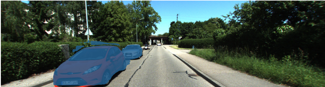
Figure 4.10: Segmentation of moving vehicles, in blue, in sequence 11_360.
