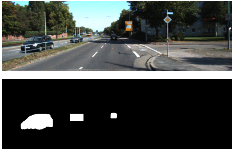
Figure 4.4: Example of a non-perfect ground truth mask, as the moving car only has the corresponding bounding box, and not the actual shape of the vehicle.
