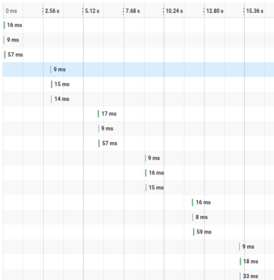
Figure 5.5: Response time for HTTP request in Raspberry
