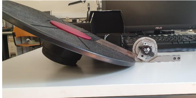
Figure 3.10 - Balance board maximum tilt measurement with protractor.
