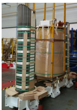
Figure 3 - a) Magnetic core structure and one of the phases mounted in the central leg of the magnetic core (from an experimental setup transformer, courtesy of Efacec) ; b) transformer's magnetic core with primary and secondary windings (adapted from [11])
