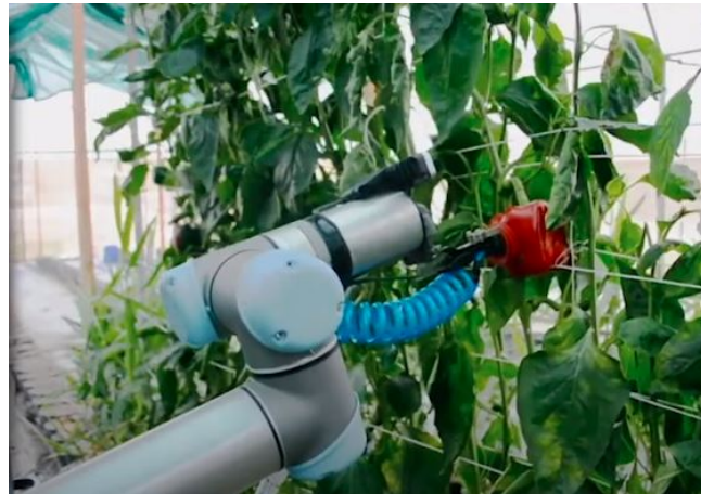
Figure 2.7: Sweet Pepper Harvester - Grip The Pepper - Adapted From The Video by Lehnert et al. [4]
