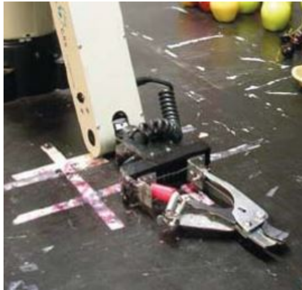
Figure 2.4: Integrated Gripper And Cutter For Harvesting Greenhouse Products - Adapted From [1]
