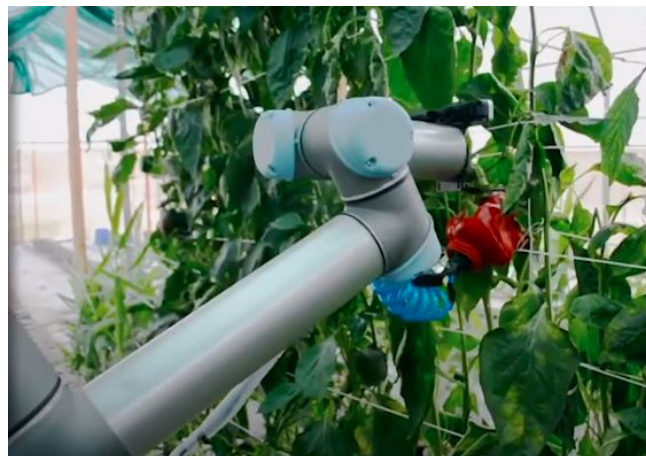
Figure 2.8: Sweet Pepper Harvester - Cut The Stem - Adapted From The Video by Lehnert et al. [4]
