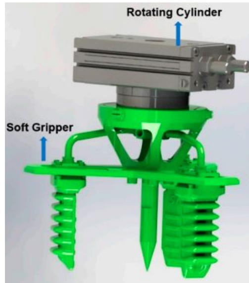
Figure 2.10: Mushroom Harvester End-Effector - Adapted From [6]
