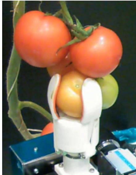
Figure 2.6: Rotational Plucking Gripper - Adapted From [3]
