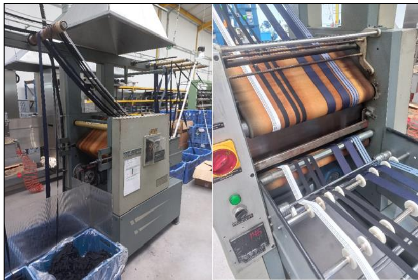
Figure 18. One of the calender machines used in IMPETUS for the elastics.
