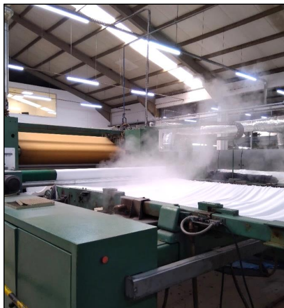
Figure 12. Sanforizing machine used in ACATEL.
