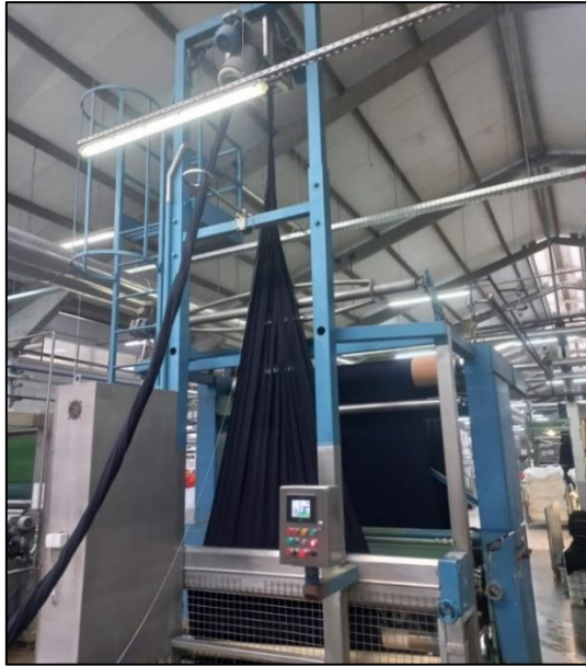
Figure 11. Machine that squeezes the fabric in ACATEL.
