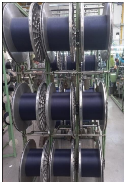
Figure 16. Warping beams that come out of the warping machine.
