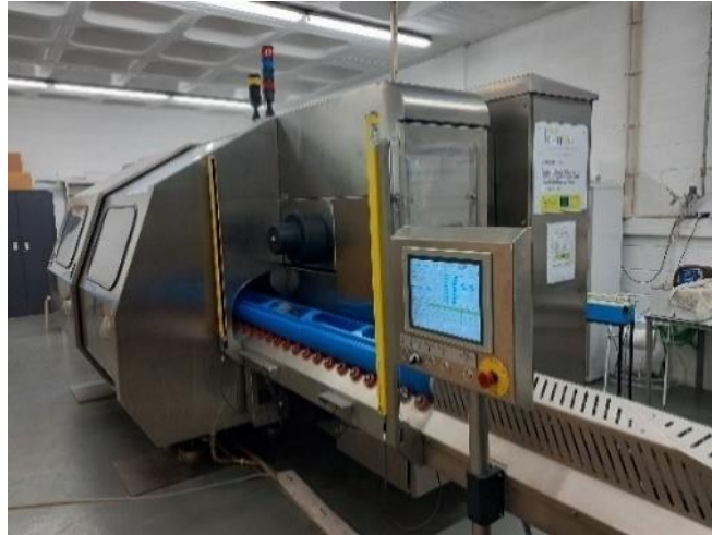
Figure 8. Pilot-scale high hydrostatic pressure equipment (Hiperbaric 55, Burgos, Spain). (Source: Author).
