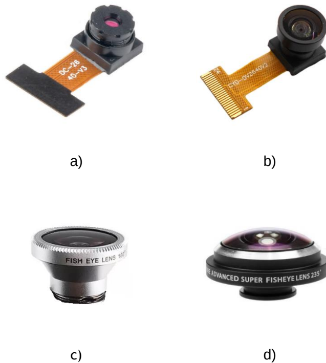
Figure 3.3 - Lenses used in the experimental tests, a) 66.5^\circ lens, b) 160^\circ lens, c) 180^\circ lens, d) 235^\circ lens.
