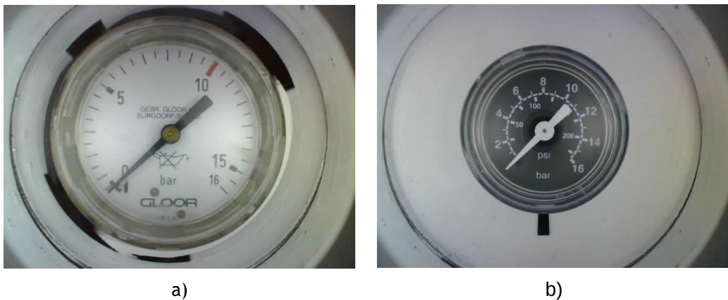
Figure 4.1 - Gauge images used to develop algorithm, a) white background gauge result, b) black background gauge result.
