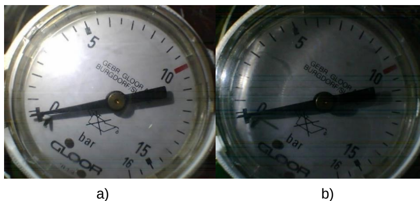
Figure 3.7 - Light technics testing, a) bright field, b) dark field.
