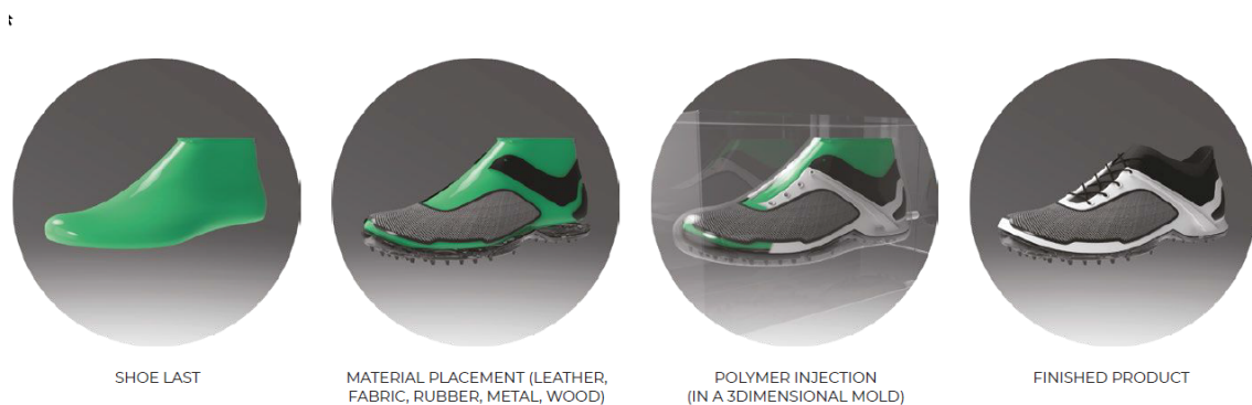
Figure 2.8: 3D Bonding Process. Retrieved from [6]
