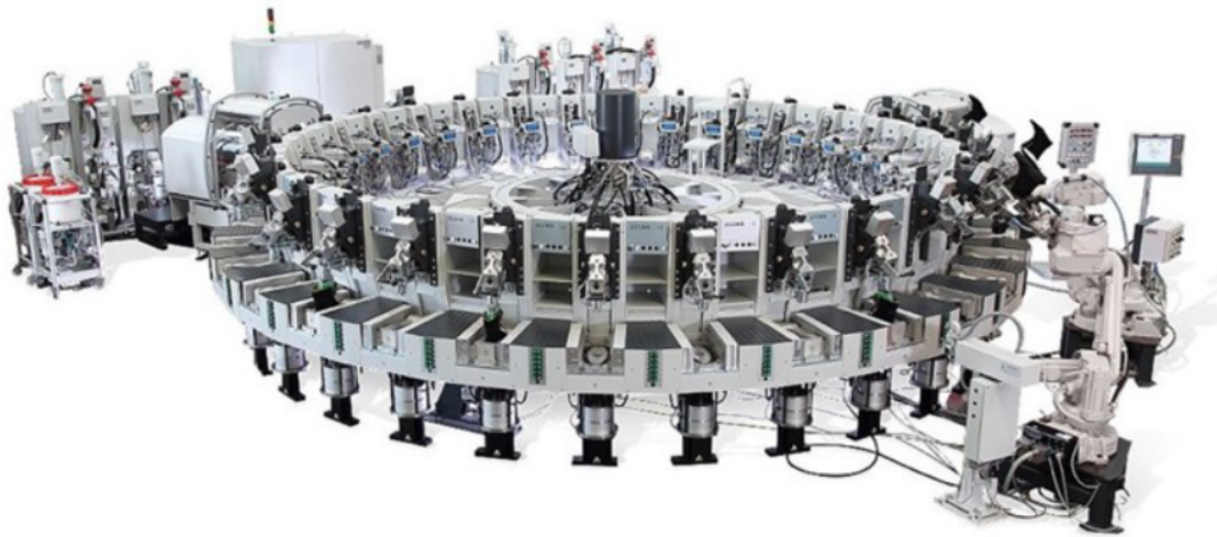
Figure 2.4: Desmas's Injection rotating machine. Retrieved from [3]
