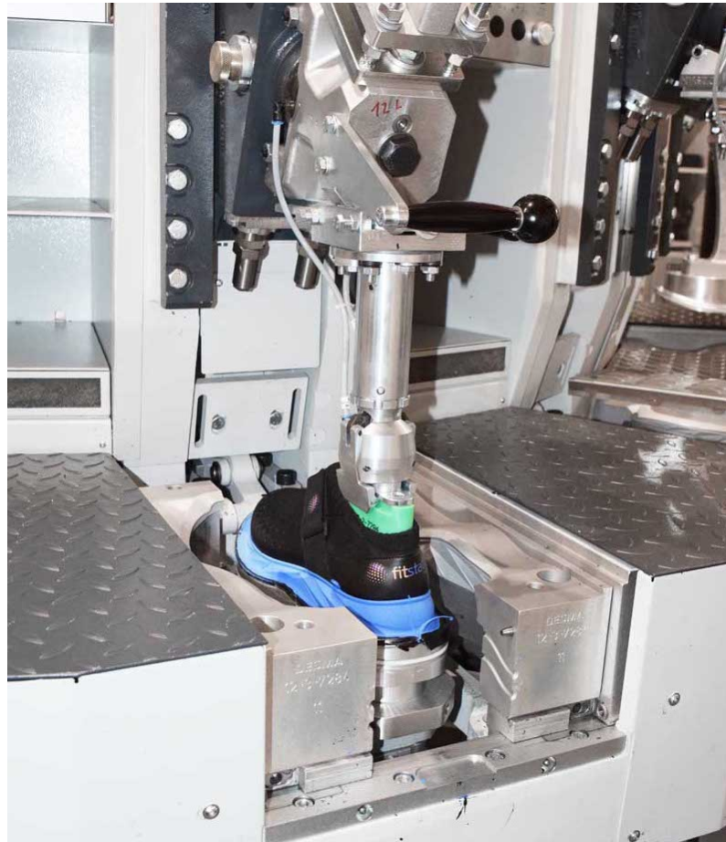
Figure 2.6: Mould of the Desmas's Injection Machine. Retrieved from [5]
