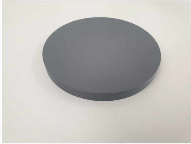
Figure 4.8: Calibration disk (Radius/Width: 100 mm / 10mm)
