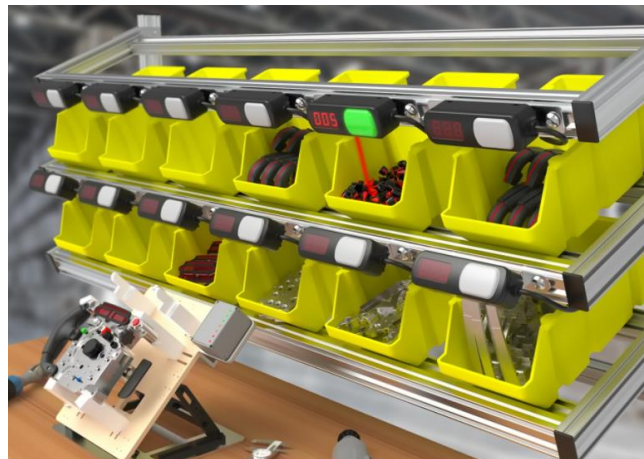
Figure 11: Functioning of a pick-by-light system (BannerEngineering, n.d.).
