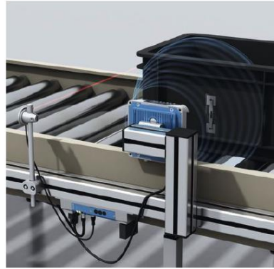
Figure 14: RFID reader installed in a roller conveyor (Dastres, Soori and Asamel, 2022).
