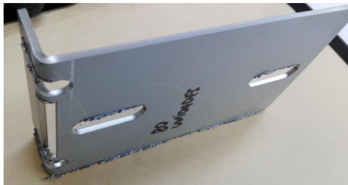
Figure 17: Non-compliant part due to excessive burr.
