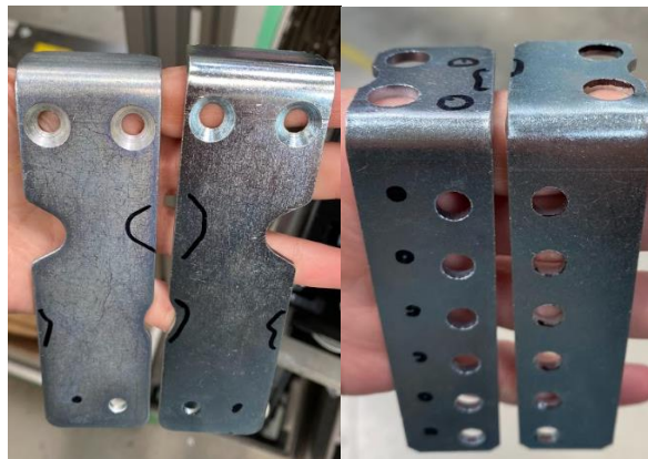
Figure 47: Examples of pairs of left/right parts that would easily be transformed into a unique part.
