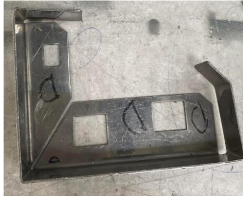
Figure 19: Poka-Yoke system used in P41 for screws alignment.
