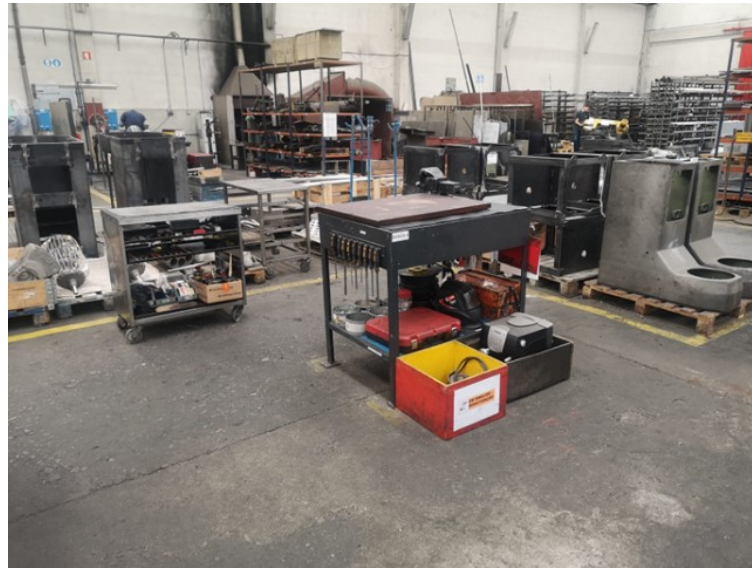
Figure 13 – Maintenance space after 5s action
