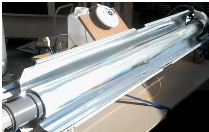
Figure 10 - Compound parabolic collector used in solar disinfection (adapted from Gutiérrez-Alfaro et al., 2018).
