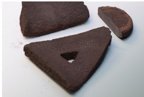
Figure 2.11: Moonbase segment made of regolith. Source: ESA (2017)
