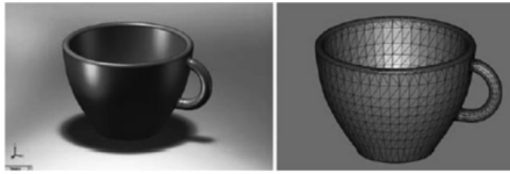
Figure 2.1: CAD model (left) and STL file (right). Source: Ian Gibson and Stucker (2015)
