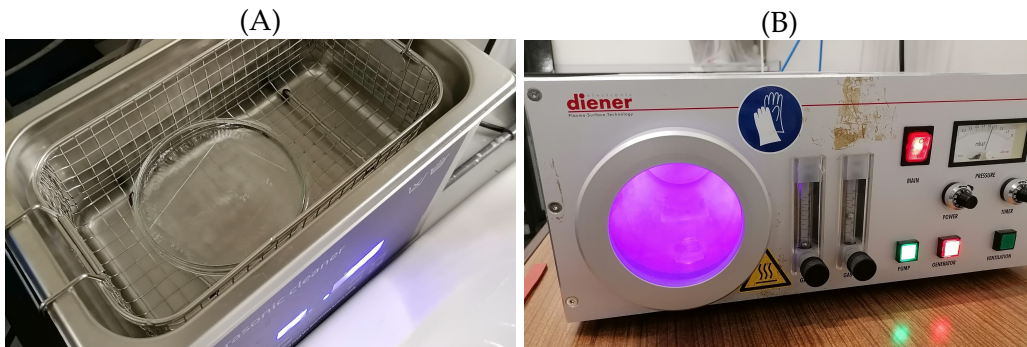
Figure 2.13: (A) ultrasonic cleaning of the glass microscope slide and (B) plasma bonding of the slide and the PDMS layer.
