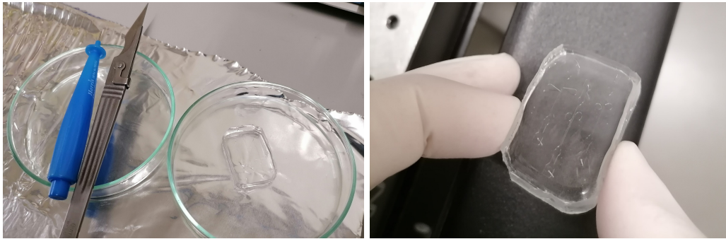
Figure 2.12: Cut, peeled and punctured, cured PDMS layer.
