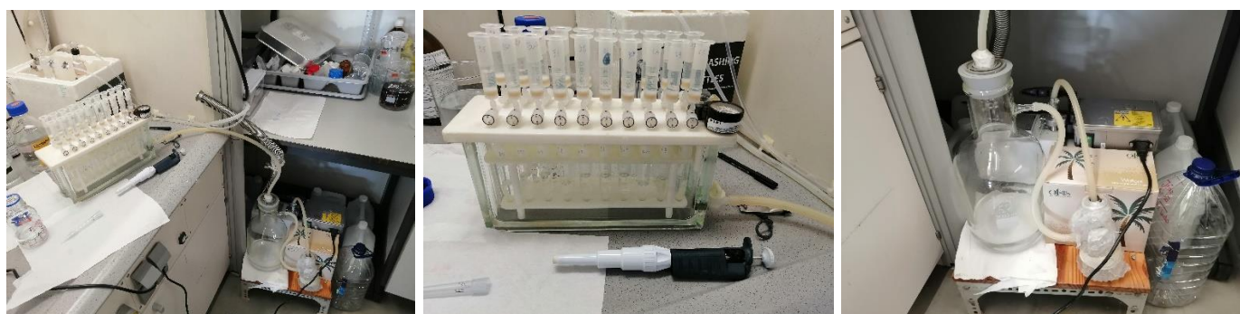
Figure 6. Experimental setup for SPE assays. Left – full setup; Middle – closeup of extraction manifold (with cartridges and tubes in place); Right – closeup of liquid trap containers and pump
