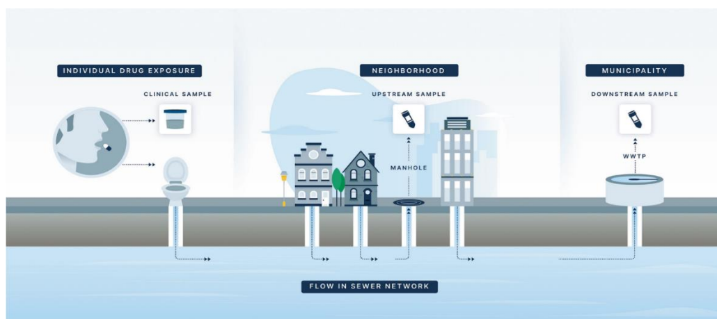
Figure 3. Possible WBE sample collection points and relative position on the sewage system. Reprinted from [62] with the permission of Springer Nature (open access article distributed under the terms of the Creative Commons CC BY license)
