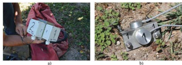
Figure 6. Accelerometers: a) piezoelectric (tower) and b) MEMs (conductor).
