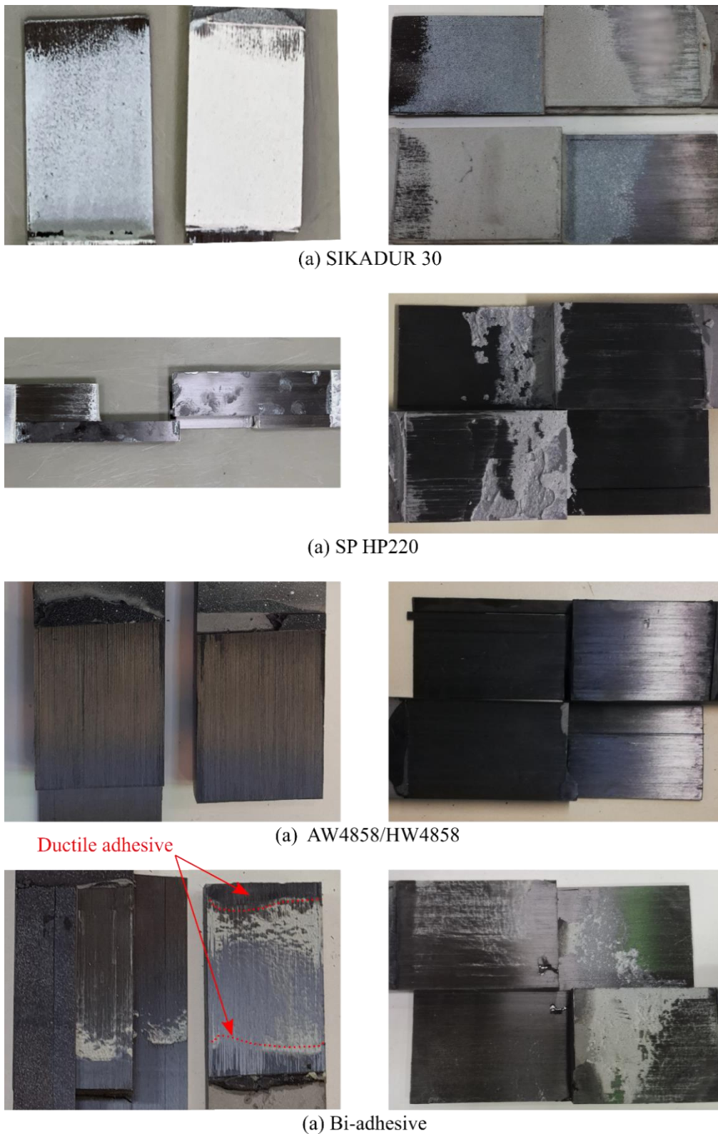
Figure 4-7: Typical failure mode for DSJ specimens: (a) SK30 adhesive, (b) AW4858/HW4858, (c) SP, and bi-adhesive.
