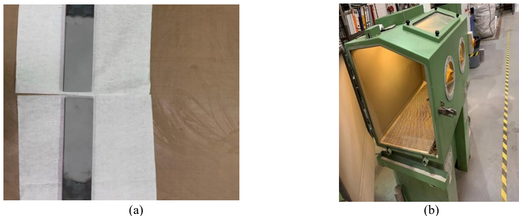
Figure 3-5: Sand blasting of the steel bars: (a) sand blasted steel bar; (b) sandblast machine.
