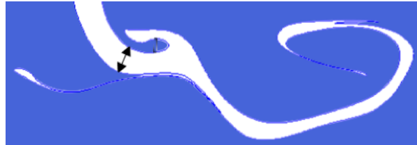
Figure III.25 Identification of zones of the flow interface: “inside” (arrow, white zone) and “outside” (blue zone).
