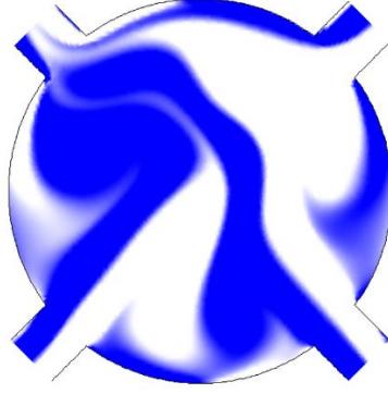
Figure IV.8 Oscillation of the NETmix jets.
