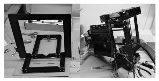
Fig. 6. Assembling the 3D printer
