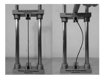
Fig. 8. Using the buckling model
