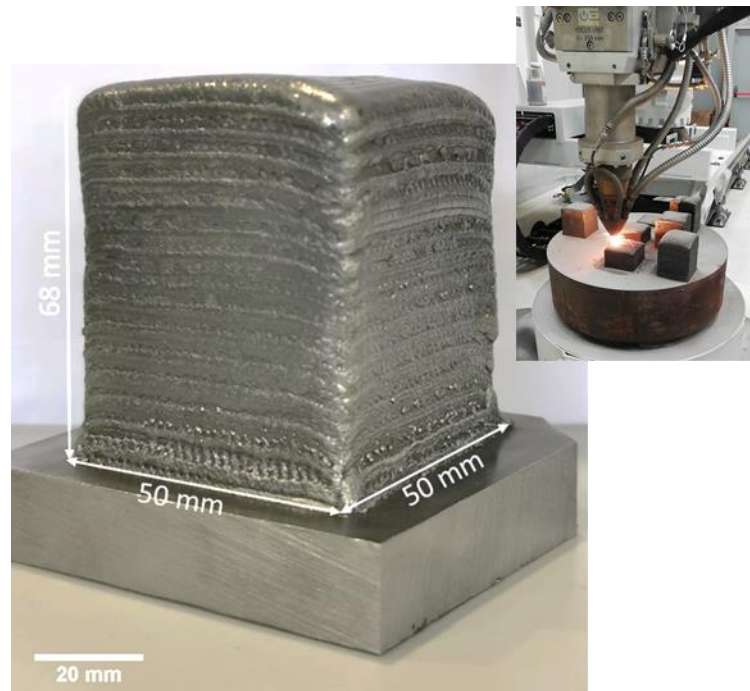
Figure 3. Bulk produced by direct laser deposition (DLD) using Inconel 625 powder deposited on 42CrMo4 steel substrate.
