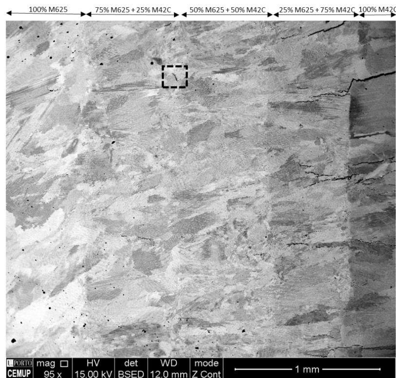
Figure 2. Microstructural evolution across the longitudinal section of the FGM specimen, SEM/BSE image.
