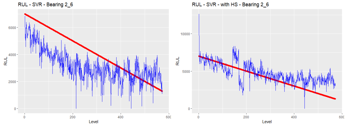
Figure 23: RUL of bearing 2_6. In the right is the model that considers the HS identification.
