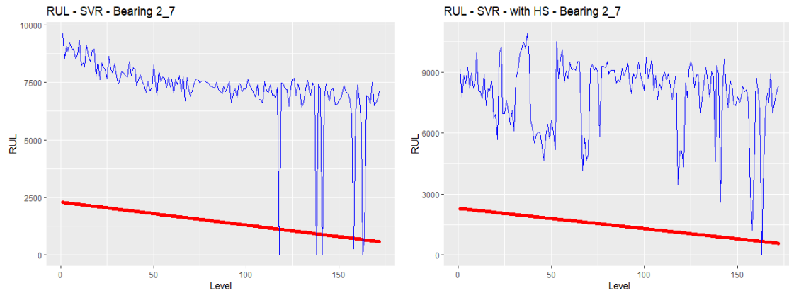
Figure 24: RUL of bearing 2_7. In the right is the model that considers the HS identification.
