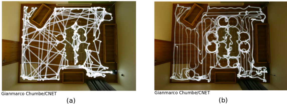
FIGURE 1.2: Comparing vacuum cleaner robots in the same environment: (a) shows the trajectory of a robot that does not build a model of the environment. (b) shows the trajectory of a robot that builds a map using an on-board range sensor. Source: [3]
