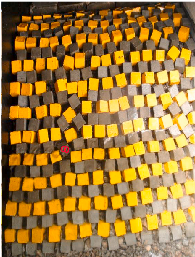
Fig. 7. Example of test results showing a cube (marked in red) that fall into the gap of the lower row due to lack of overlapping. Courtesy of Almeida (2013).
