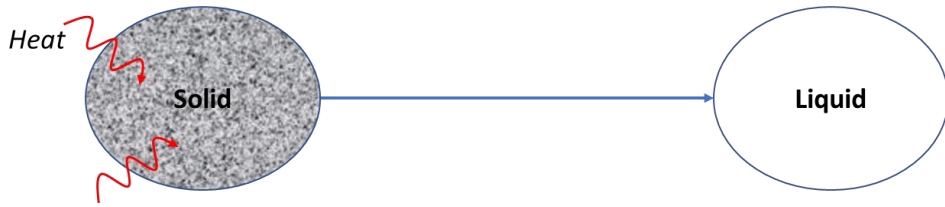
Figure 1.1 - Phase change material melting as it absorbs heat from the environment at the melting temperature.
