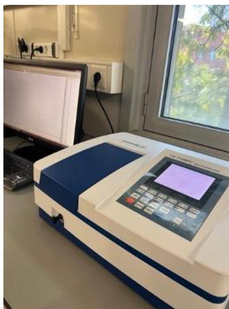
Figure D 1. 2- Spectrophotometer used to obtain the absorption spectrum - UV-3100PC Spectrophotometer.
