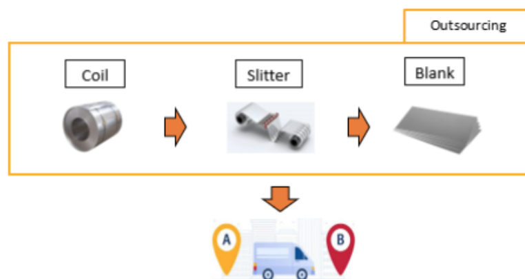
Figure 4.20: Current outsourced production for the part in assessment (re-created after [ 15 ])
