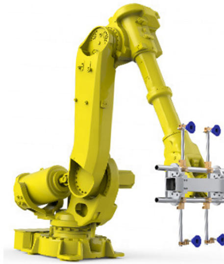
Figure 4.5: Robot (R1) and suction cups grip [53]
