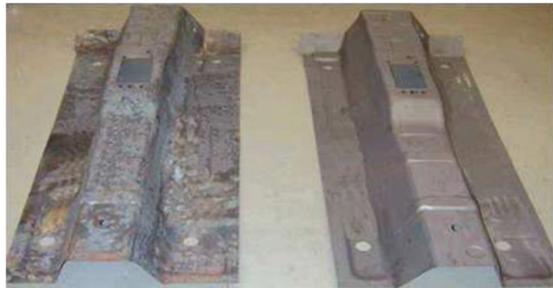
Figure A.6: VW Passat transmission tunnel hot stamped using: (left) uncoated blank causes scales; (right) coated blank has no scale problems [45]
