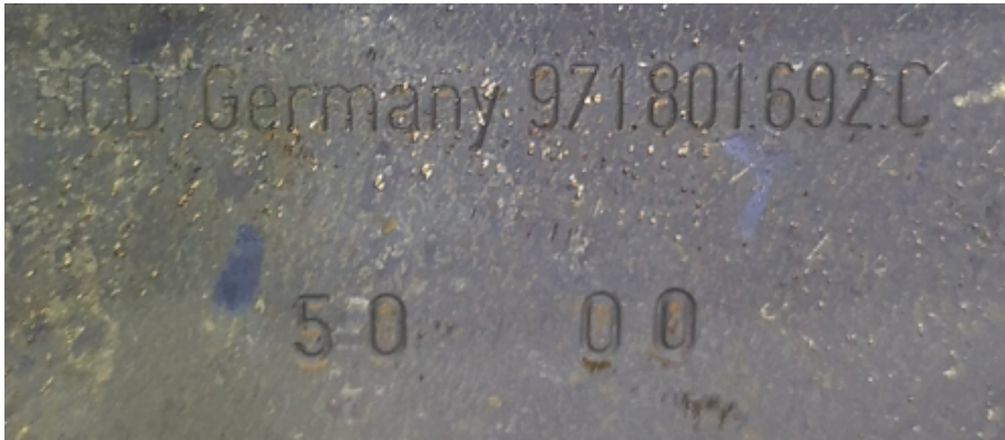
Figure 4.7: Traceability engravings on the parts
